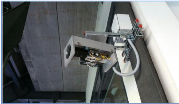
1. Mount the Camera to the camera mount in the cabinet using four screws to hold the camera in place. Insert the screws from the outside and tighten snugly with a Phillips screwdriver.
