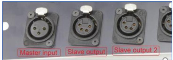
The Master Server Trigger Cable consists of an SDR connector, an XLR 4-pin connector, and an XLR 3-pin connector. Use the Master Server Trigger Cable to complete these steps:
