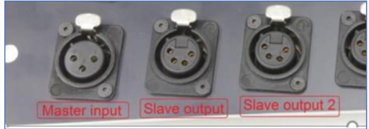
The Slave Server Trigger Cable consists of an SDR connector, and an XLR 4-pin connector. To connect the Slave Server to the Trigger Panel, complete these steps:
