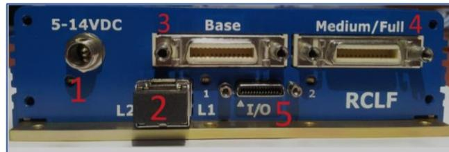
4. Connect a Camera Link Cable from the **DIGITAL I/O 1** connector on the Camera to the **Base** connector on the Extender.
